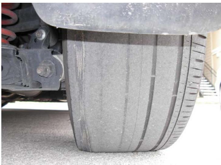
Wheels can go out of alignment causing wear to the inner tyre tread – you may not notice it, but your tyre won't give you the grip it should in the wet. Even modern cars use oil, and it is much better for the engine if you detect that the oil is low before the warning light appears.
